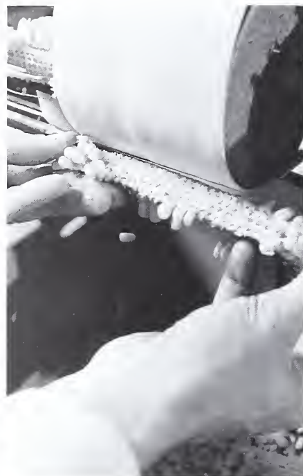
In improved system for processing sweet corn, split ears are rotated while being pushed against revolving drum. Rubbing action removes the kernels intact. The Western lab process reduces organic wastes by up to 80 percent.
