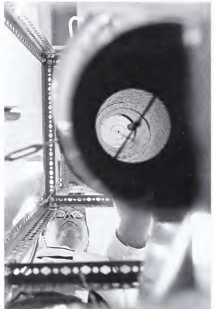
Water swirls down the inner surface of an experimental wet-wall air cleaner, washing away electrically charged particles of cotton dust. The cleaner, tested here by SRRC physicist Devron P. Thibodeaux, uses both electrostatic and inertial forces to control and remove dust in cotton gins and textile mills.
