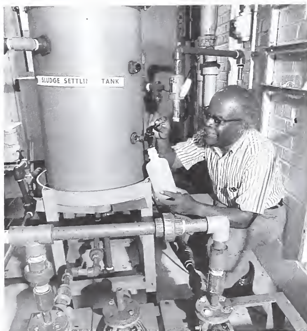
Developing a more economical process to treat sulfide-laden tannery wastes, Joseph Cooper, an ERRC research chemist, collects biosludge from settling tank. He will then examine a sample under a microscope to determine the efficacy of microbes in the anaerobic treatment system.
