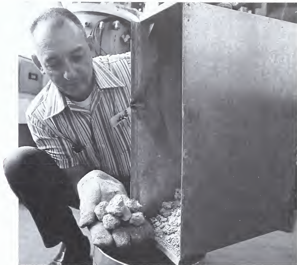
In Western lab, engineer Everett Durkee removes recycled salt left from olive processing after contaminants are incinerated. Salt can be reused during next olive season.
