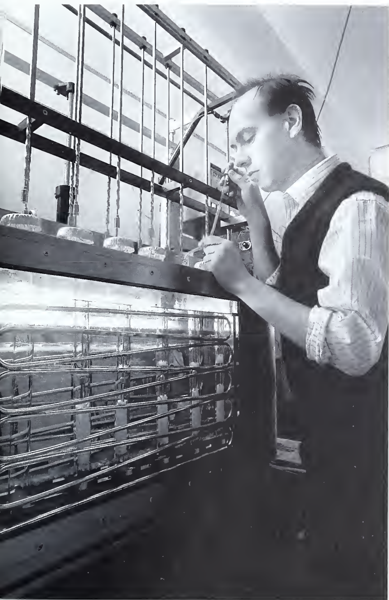
ERRC chemist Christopher Carr monitors bleaching reactions on samples of urine-stained wool.
