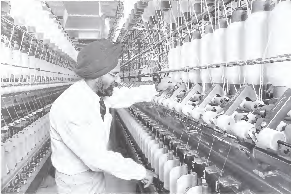
SRRC cotton technologist A. Paul Sawheny checks on patented new system to blend more cotton fiber with synthetic fibers to make fabrics that combine strength of synthetics with comfort and breathability of 100-percent cotton.
