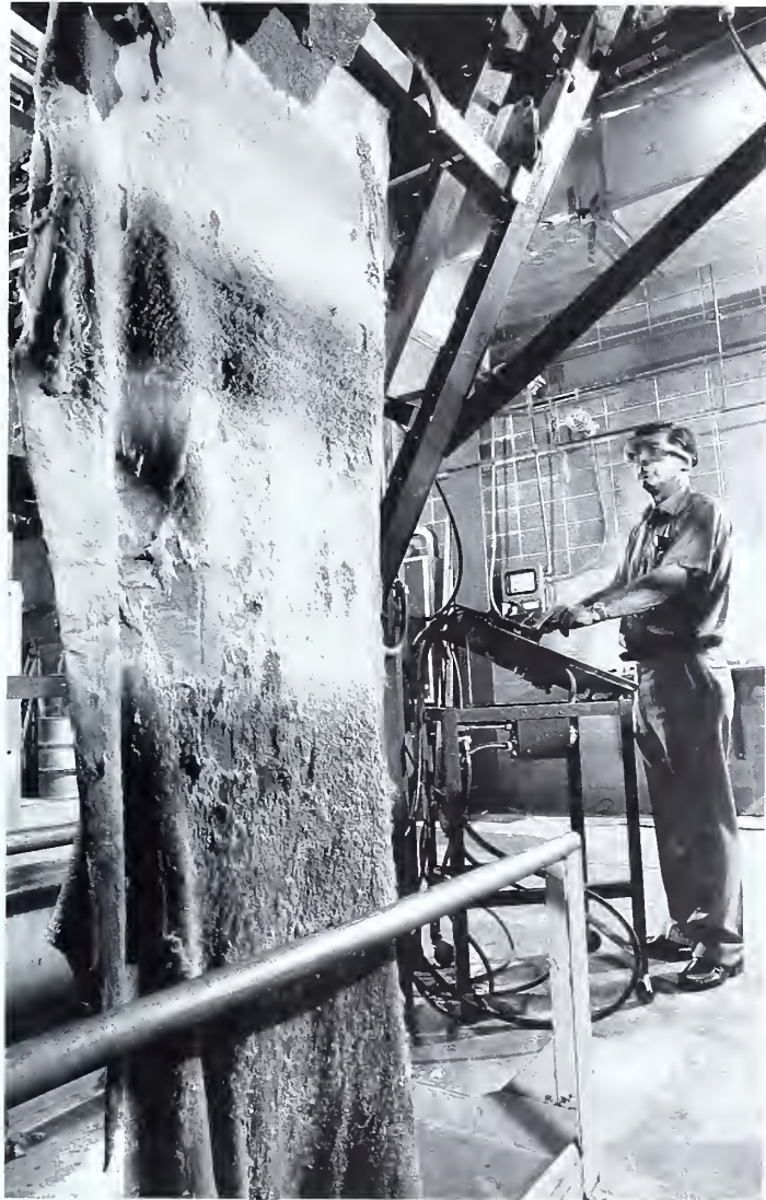
After passing through the first of three conveyors in the pilot plant for continuous beamhouse processing, a hide with hair loosened by chemicals is ready for the unhairing machine. ERRC mechanical engineer Wolfgang Heiland operates the control panel, moving the hide to the second conveyor.
