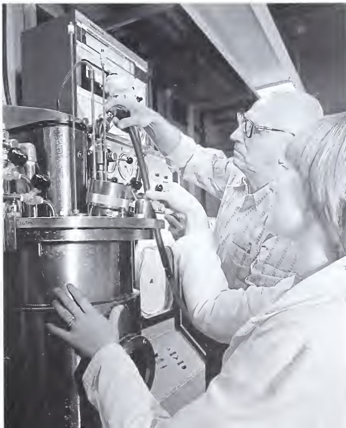
Peoria chemical engineer Patricia J. Slininger and A. A. Lagoda, engineering technician, prepare a fermentor for growing cells of Pachysolen tannophilus , an unusual yeast that can convert biomass to alcohol.
