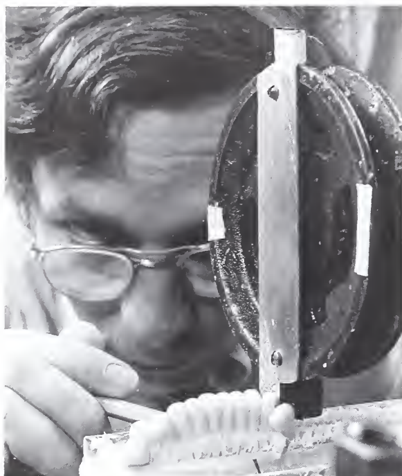
Designing new equipment and techniques to process whole kernel sweet corn, WRRC chemical engineer George Robertson determines exactly how much force is necessary to remove an intact kernel of a particular variety of corn from the cob.
