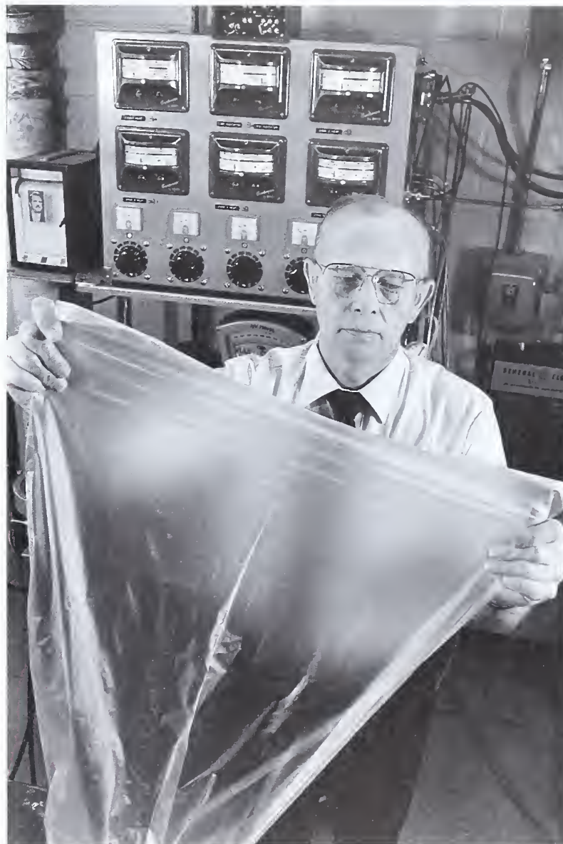
Peoria chemist Felix Otey stretches a sheet of biodegradable plastic film, made from starch and petroleum-based polymers.
