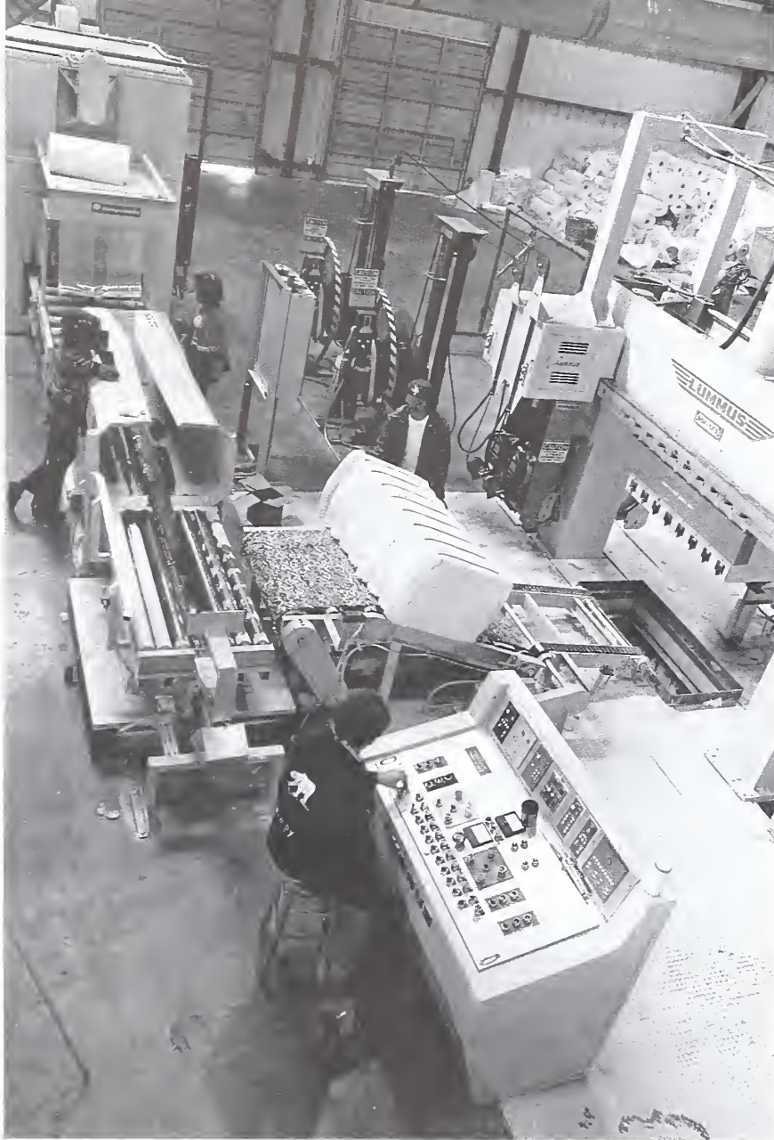
Modern cotton gin, producing 35 bales an hour, bears little resemblance to outmoded gins of World War II vintage and contains many innovations resulting from SRRC research.
