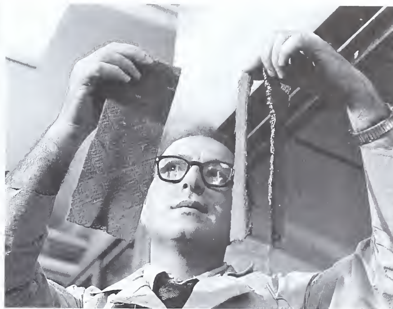
After conducting flame tests on wool, Mendel Friedman, WRRC research chemist, compares fabric on left treated with chemical flame retardant with untreated fabric on right. The treated fabric charred slightly but wouldn't ignite.
