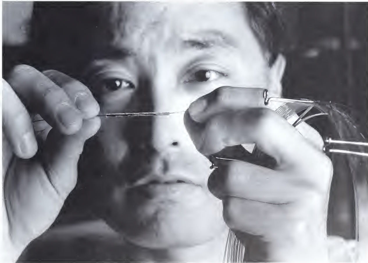
At WRRRC, Chemist Gary Takeoka prepares a chromatographic column for tests capable of detecting flavor adulterants.
