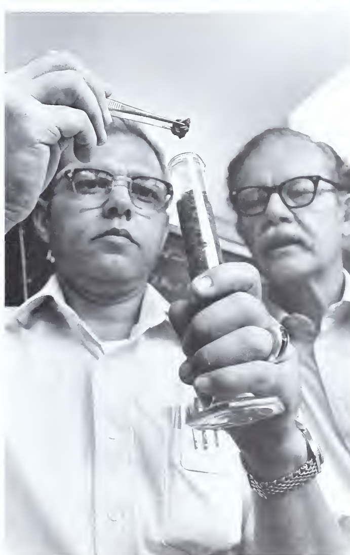
One use for artificial gravel, made by combining cellulose xanthate with soil, is to surround perforated drainage tubes to prevent clogging of holes by fine soil particles. WRRRC researchers Earl Hautala (left) and Emory Menefee developed xanthate from waste cellulose products.
