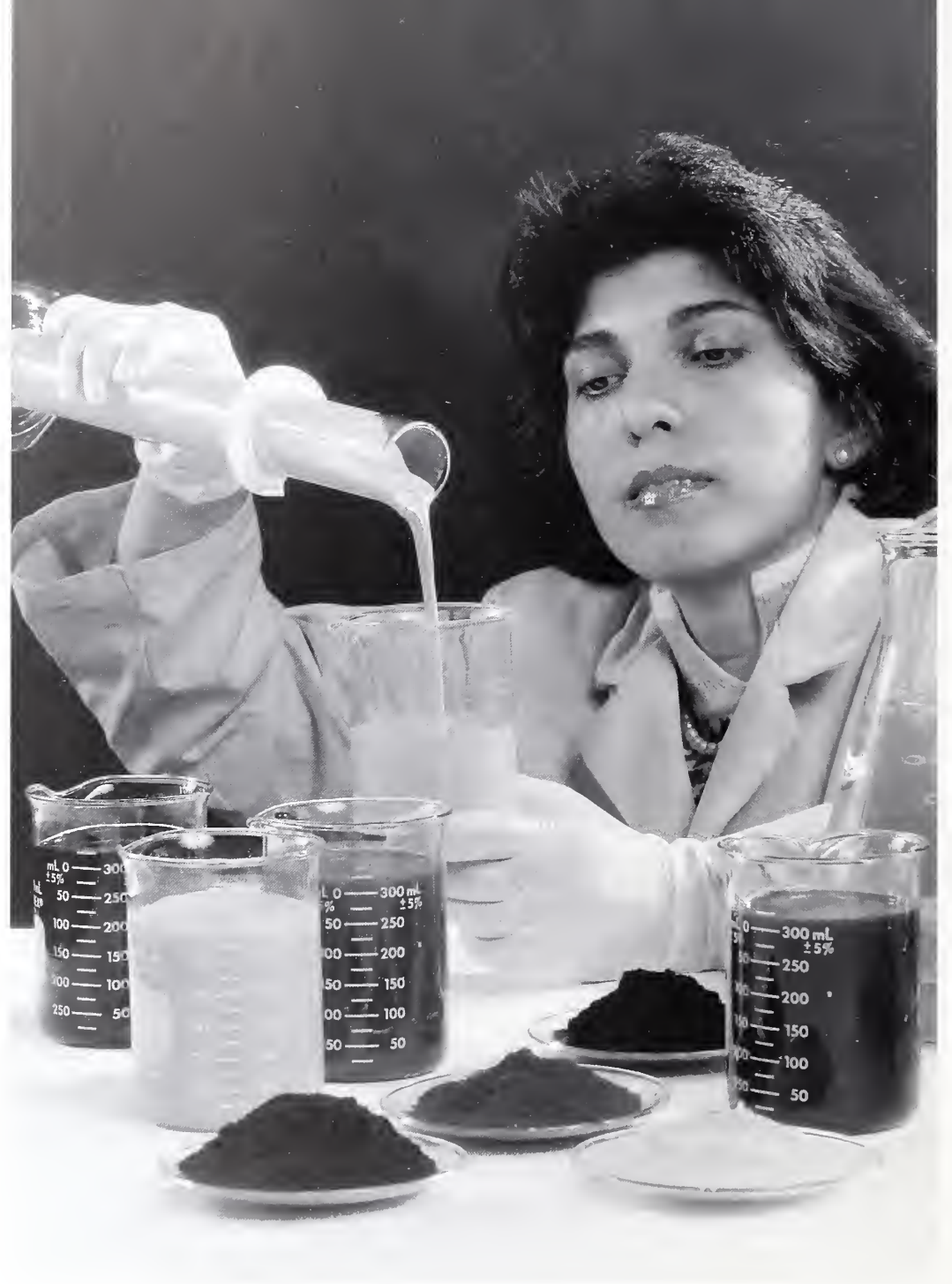
Sevim Erhan, a chemist in the Peoria center, prepares black and color newsprint inks made from 100-percent soybean oil for printing tests in the laboratory.
