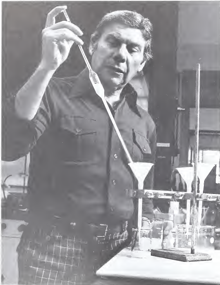
Chemist Daniel P. Schwartz tests milk for traces of the antibiotic chloramphenicol (CAP) in an inexpensive yet sensitive procedure developed by his group at ERRC. Use of the drug in dairy cattle and meat animals is illegal.
