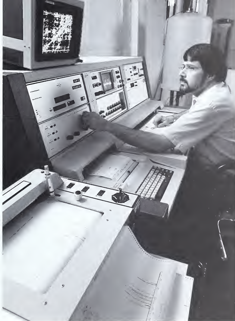
More than 40 years later, Peoria chemist David Weisleder uses magnetic resonance imaging to identify pesticides occurring in plant materials.
