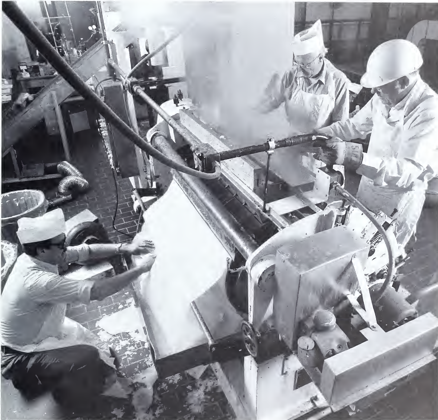
Engineers in ERRC pilot plant process mashed potatoes into a continuous sheet that can be broken up into instant potato flakes.
